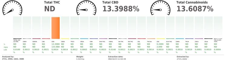
Analysis Method : SOP.T.40.039.CO Analytical Batch : DE006213POT Instrument Used : Agilent 1100 "Falcor"
